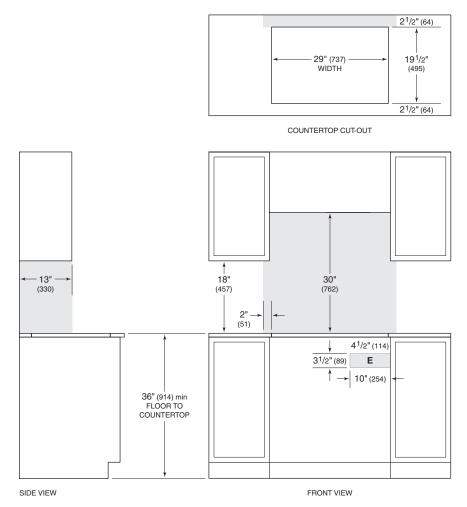
NOTE: Shaded area above countertop indicates minimum clearance to combustible surfaces, combustible materials cannot be located within this area. Electrical supply location only applies to installations with built-in oven.
