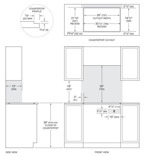
NOTE: Shaded area above countertop indicates minimum clearance to combustible surfaces, combustible materials cannot be located within this area.
