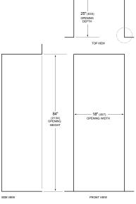
NOTE:3<sup>1</sup>/<sub>2</sub>" (89) finished returns will be visible and should be finished to match cabinetry
