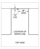
ICE MAKER DRAIN Ice maker models can be ordered with or without a drain pump. Models without a pump will drain water by gravity. A drain must be provided for all models.
