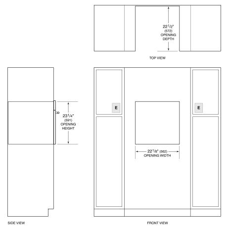
NOTE: Electrical supply must be located in adjacent cabinet within 3' (.9 m) of opening.
