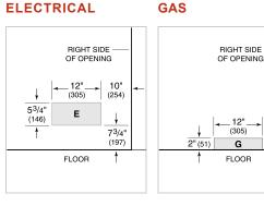
NOTE: Dimensions in parenthesis are in millimeters unless otherwise specified
