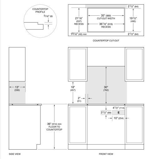
NOTE: Shaded area above countertop indicates minimum clearance to combustible surfaces, combustible materials cannot be located within this area. Electrical supply location only applies to installations with built-in oven. Outside corner radius 7/16" (11).
