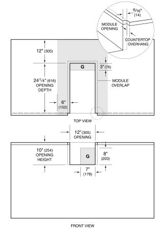
NOTE: Shaded area above countertop indicates minimum clearance to combustible surfaces, combustible materials cannot be located within this area. An insulating liner is not required.
