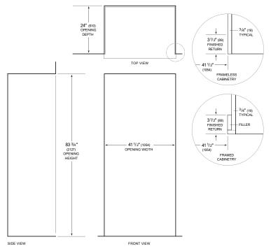
OTE: 31/2" (89) finished returns will be visible and should be finished to match cabinetry
