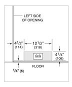
**NOTE:** The electrical outlet must be positioned with the grounding prong to the right of the thinner blades.
