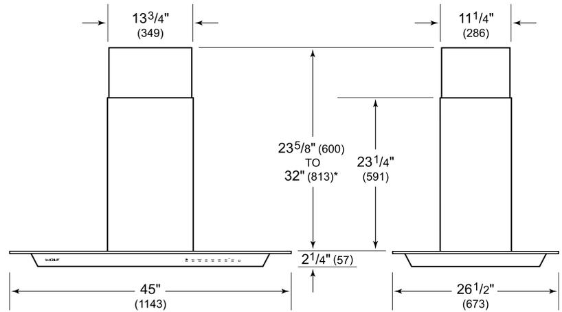
\*51<sup>1</sup>/<sub>8</sub>" (1299) to 59<sup>1</sup>/<sub>2</sub>" (1511) with accessory flue extension.
