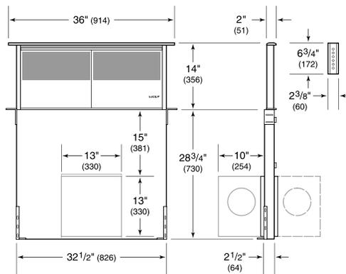
**NOTE:** Shown with front mounted internal blower with 6" (152) round discharge, dashed line represents rear mount.
