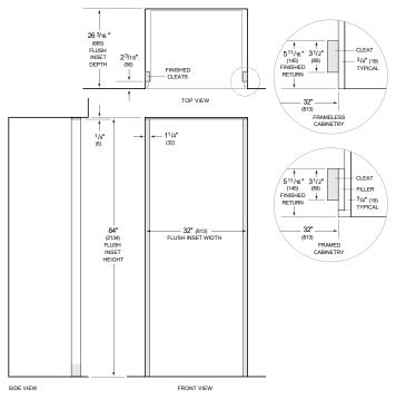
$NOTE: 3^1/z^*(89) \ finished \ returns \ and \ shaded \ areas \ will be \ visible \ and \ should \ be \ finished \ to \ match \ cabinetry \ Shaded \ line \ represents \ profile \ of \ unit \ brift/a" (19) \ panel.$
