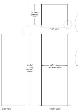
NOTE: 3<sup>1</sup>/2" (89) finished returns will be visible and should be finished to match cabinetry Shaded line represents profile of unit.
