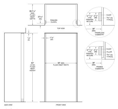
NOTE:  $3^{1}/2^{n}$  (89) finished returns and shaded areas will be visible and should be finished to match cabinetry. Shaded line represents profile of unit with  $3^{1}/4^{n}$  (19) panel.
