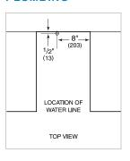
**ICE MAHINE DRAIN** Ice machine models can be ordered with or without a drain pump. Models without a pump will drain water by gravity. A drain must be provided for all models.
