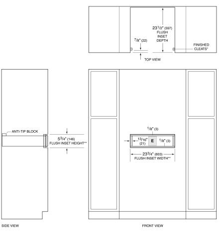
\*Will be visible and should be finished to match cabinetry. \*\*Dimension provides minimum reveals.
