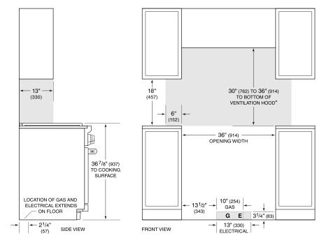
\*Without ventilation hood, 36" (914) minimum clearance countertop to combustible materials, 44" (118) for charbroiler. NOTE: Shaded area above countertop indicates minimum clearance to combustible surfaces,
