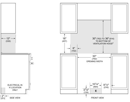
\*Without ventilation hood, 36" (914) minimum clearance countertop to combustible materials. NOTE: Shaded area above countertop indicates minimum clearance to combustible surfaces. Combustible materials cannot be located within this area.
