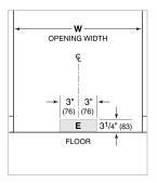
**IMPORTANT NOTE:** Adjacent countertops must be at least 35 7/8" for flush installation to top of unit.
