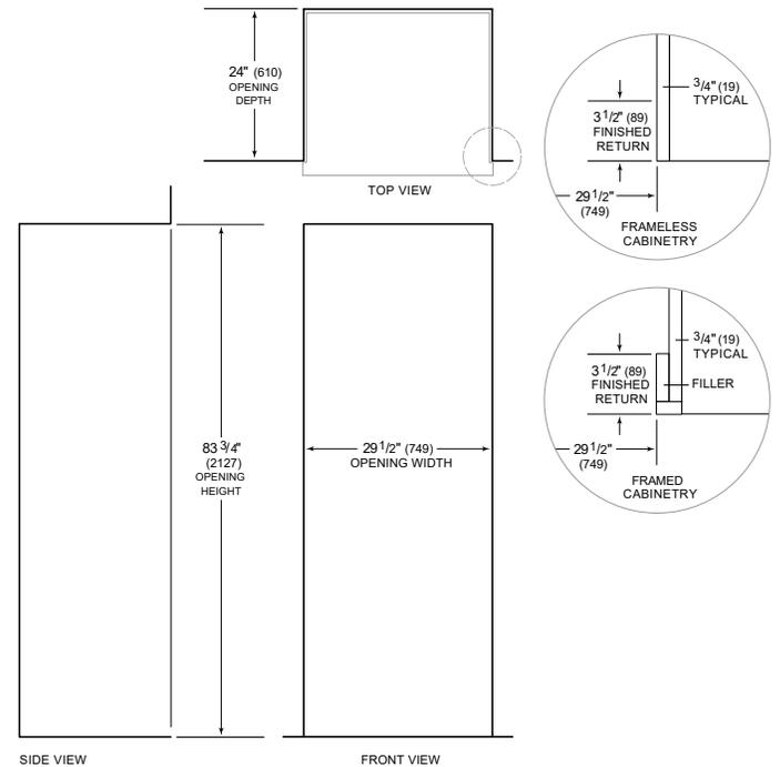
**NOTE:** 3 1/2" (89) finished returns will be visible and should be finished to match cabinetry. Shaded line represents profile of unit.
