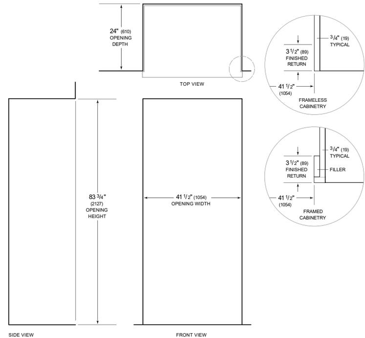
NOTE: 3 1/2" (89) finished returns will be visible and should be finished to match cabinetry. Shaded line represents profile of unit.
