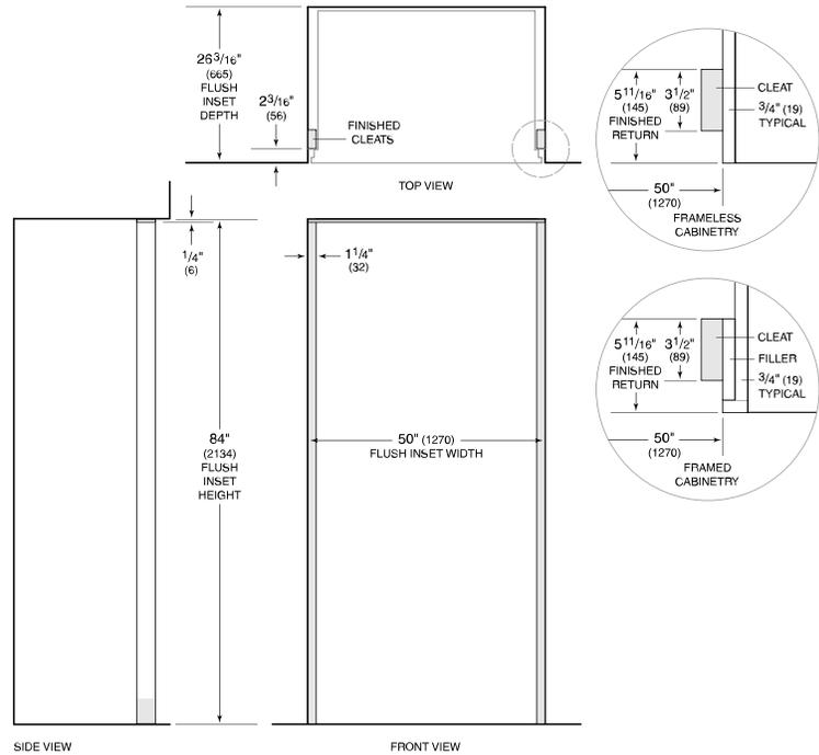
**NOTE:** 3/2" (89) finished returns and shaded areas will be visible and should be finished to match cabinetry. Shaded line represents profile of unit with 3/4" (19) panel.
